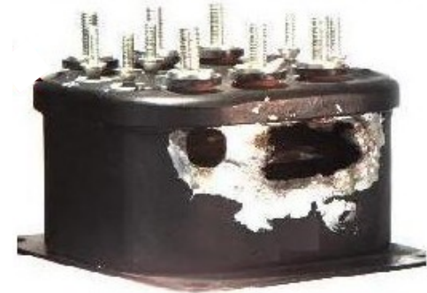
Davy, G., (Northrop Grumman Electronic Systems), “Relay Failure Caused by Tin Whiskers,”
